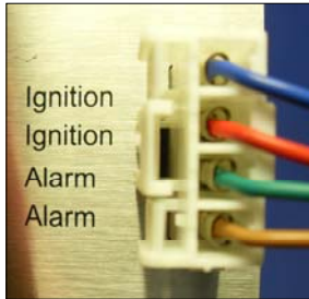
Figure 4: Ignition Interlock Relay & Alarm Contact Pair
