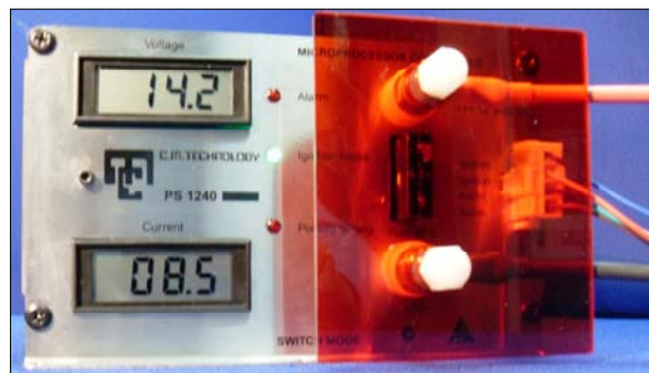
Figure 1: The PS1240 On-Vehicle Battery Manager
