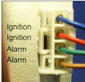
Figure 4: Ignition Interlock Relay & Alarm Contact Pair
